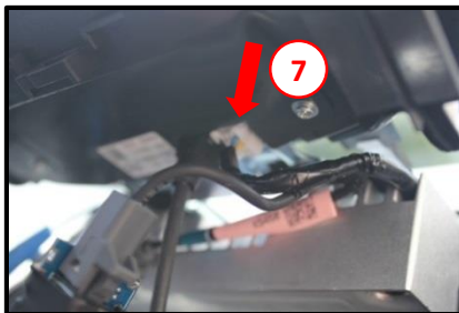
7. Unplug the factory 8-pin male display power harness and plug it into the female 8-pin MZ-72F power harness. Plug the 8-pin male connector of the MZ-72F power harness back to the display. Connect the 8-pin (with one red wire) header to the MZ-72F module. (see diagram on page 1)
