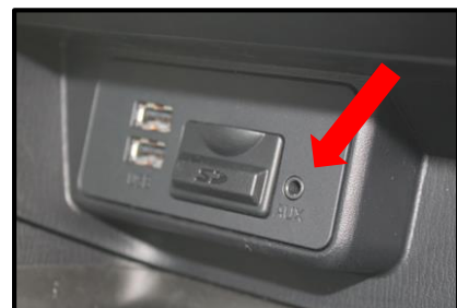
5. Using a 3.5mm to RCA cable, plug the audio output to the audio input of the vehicle.
