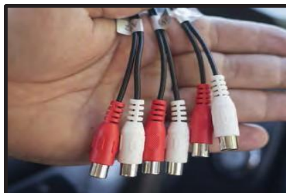
4. Plug the Audio devices to the RCA audio inputs.
