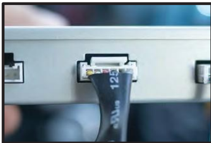
1. Plug the 6-Pin Video Harness to the main interface module. This allows 3 video inputs.
