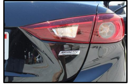
8. Run a wire from the reverse light +12V lead to the front of the vehicle and connect to the cam trigger wire (Green) of the MZ-72F harness.
