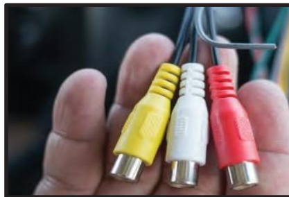
2. Plug the Video devices to the RCA video inputs. See right for video input description.
