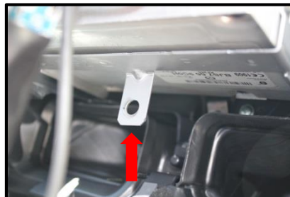
2. Remove 10mm screw to remove the radio.
