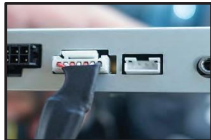
3. Plug the 6-Pin Audio Harness to the main interface module. This allows 2 audio inputs and 1 audio output.
