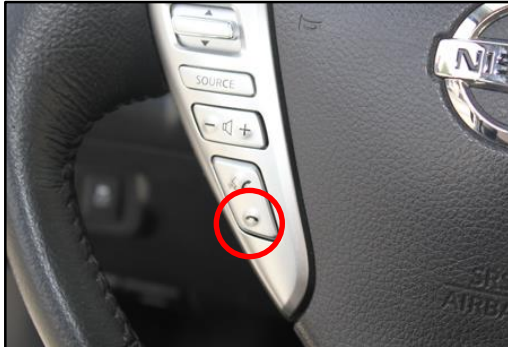
Press and hold the END CALL button for 2 to 3 seconds to toggle VIDEO IN.
